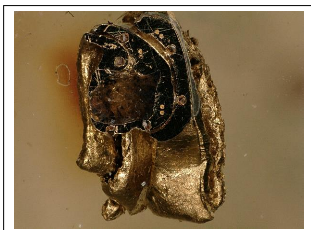
Light microscope (Keyence VHX-6000) image of a Bernstein gold sample embedded in resin. Note the irregular surface and the measuring points of the LA-ICP-MS..
