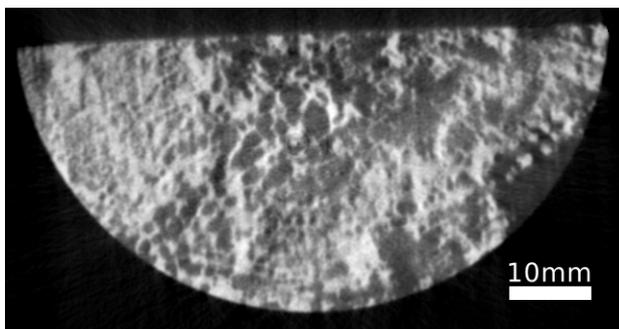
Fig. 1. Example of the CT reconstruction of the Galena mineral (lead-sulfide in the quartz matrix) with mean density of 8.3g/cm<sup>3</sup> (73% of the pure lead).
