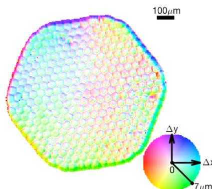
Figure 1: Capillary pointing accuracy measured with edge scans and a medipix detector. Color indicates local pointing deviation, magnitude and direction relative to focus center. Scale bar refers to positions on optic exit.
